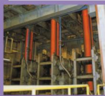
連続 casting 設備 Completely vertical type bloom caster
